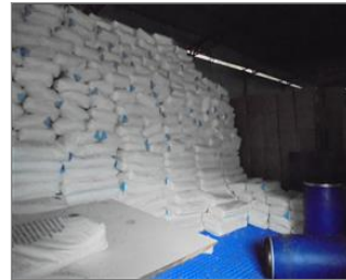
Photo of non-conformity Salt sacks stacked in excessive height.JPG
